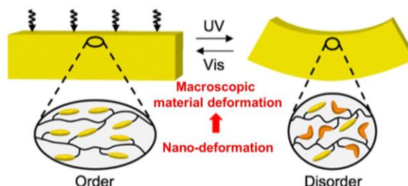
Figure 1. Light-induced deformation of crosslinked photochromic liquid-crystalline polymers
